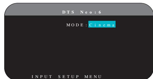
When DTS Neo:6 is selected as the default surround mode on the INPUT SETUP menu, there are additional option settings and parameters available to optimize the surround decoding for various types of recordings, music or movie soundtracks. DTS Neo:6 uses matrix decoding algorithms to derive a center channel and surround channels from 2-channel source material.
