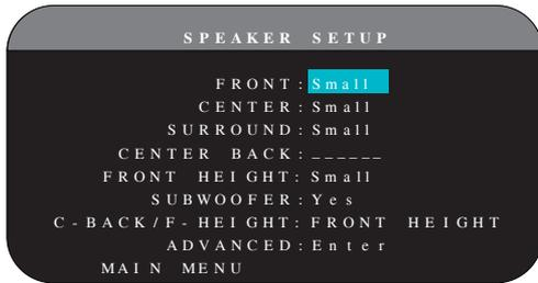
The SPEAKER SETUP menu is used to configure the RSP-1572 for use with your specific loudspeakers and to determine the bass management configuration as described in the previous overview. The menu is accessed from the MAIN menu.
