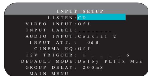
The INPUT SETUP menu configures the source inputs and is reached from the MAIN menu. The screen provides the following options, selected by placing the highlight on the desired line using the Up/Down buttons:
