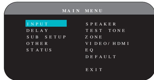
The MAIN MENU provides access to OSD screens for various configuration options. MAIN MENU is reached by pressing the RCVR/SETUP button on the remote. To go to the desired menu, move the highlight using the Up/Down and Left/Right buttons on the remote and press the ENT button. Press the RCVR/SETUP button again to cancel the display and return to normal operation.
