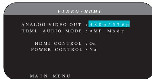
The VIDEO/HDMI menu deals with the configuration of the HDMI output for high-definition video display devices. See the Video Inputs & Outputs section of this manual.
