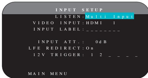
When the MULTI INPUT source is selected on the INPUT SETUP menu, the available options change to reflect the fact that these inputs are direct analog inputs and bypass the unit's digital processing. The INPUT, CINEMA EQ, DEFAULT MODE and GROUP DELAY options are not available since these are all digitally implemented features.
