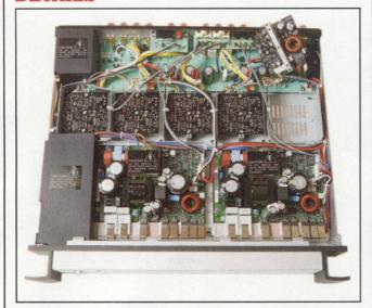
Like an electronic jigsaw everything inside the RMB-1077's chassis slots neatly into place, including the switch-mode power supply at the front and modular PWM amplifiers located in separate compartments. One of the ICEpower modules – the real heart of the amplifier – is lifted clear for clarity. At the back you can see the inductors (coils) that form part of the final analogue filter network.
