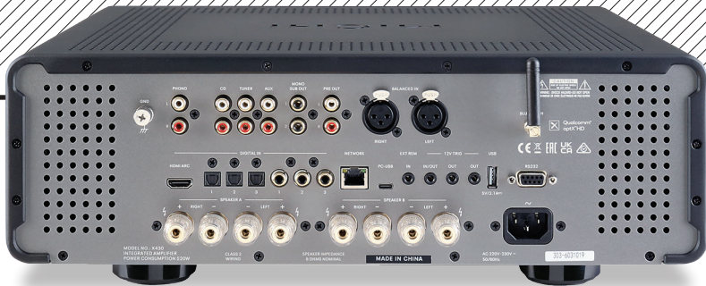
ABOVE: Switched A/B speaker binding posts and variable preamp outputs, on RCAs, are joined by MM phono and four line inputs (one balanced on XLR). Digital inputs include three optical/coaxial, USB-C, HDMI ARC and wireless BT. Ethernet is for control
