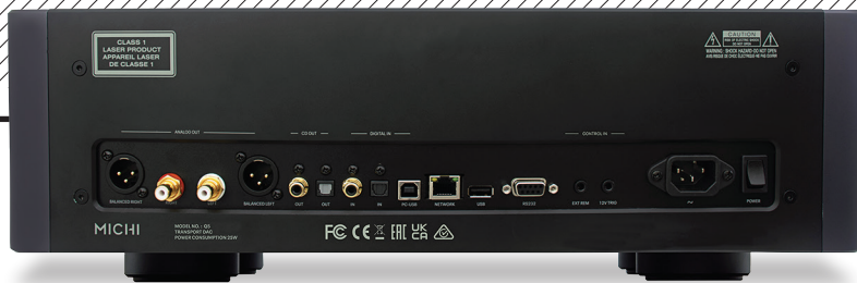
ABOVE: Balanced XLR and unbalanced RCA outputs are joined by optical and coaxial outs (CD transport), optical and coaxial (192kHz/24-bit) and USB-B (384kHz/32-bit, DSD256) inputs, Ethernet (artwork, firmware), USB (firmware), and control/RS232 ins
