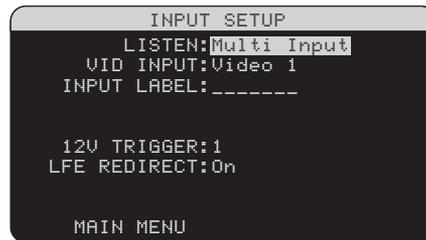
When the MULTI INPUT source is selected on the INPUT SETUP menu, the available options change to reflect the fact that these inputs are direct analog inputs and bypass the RSX-1056's digital processing. The INPUT, CINEMA EQ, and DEFAULT MODE options are not available since these are all digitally implemented features.
