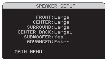
The SPEAKER SETUP menu is used to configure the RSX-1056 for use with your specific loudspeakers and to determine the bass management configuration as described in the previous overview. The menu is accessed from the MAIN menu.
