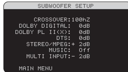
The SUBWOOFER SETUP menu allows selection of the master subwoofer crossover frequency and independent adjustment of subwoofer level for each surround mode.
