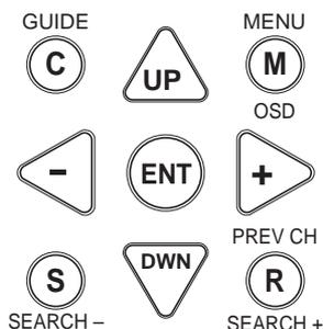
**MENU/OSD button:** Press to display the SYSTEM STATUS screen. From the SYSTEM STATUS screen, press the ENTER button to display the MAIN MENU screen which has links to all other menus. If a menu is already visible, push this button to cancel the display. The MENU button on the front panel provides the same function.
