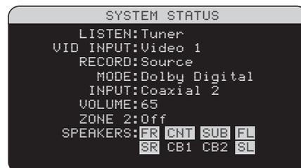
The SYSTEM STATUS menu provides a snapshot of the current system settings and a starting point for reaching all other screens and menus. This screen appears when you press the remote MENU/OSD or front panel MENU button and displays the following information:
