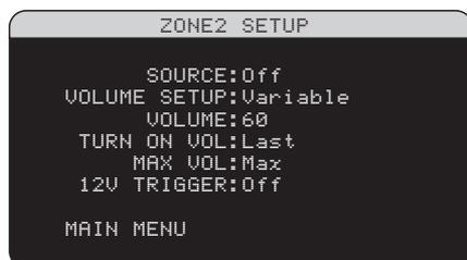
The ZONE 2 SETUP menu provides settings and configuration options related to the operation of Zone 2. This menu is reached by highlighting the ZONE 2 line on the MAIN menu and pressing ENTER.
