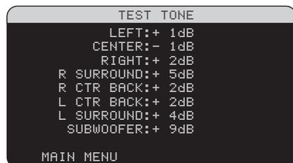
This menu uses filtered pink noise test tones to set equal volume levels for all speakers (left front, center, right front, right surround, center back, left surround, and subwoofer) to ensure proper surround sound reproduction. Setting the output levels using the test procedure provides the most accurate adjustment so that digital surround sound material will be reproduced as it was intended and is a critical step in calibrating the system.
