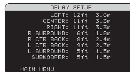
The DELAY SETUP menu, which is reached from the MAIN menu, allows you to set the delay for individual speakers. This ensures that the sound from each speaker arrives simultaneously at the listening position, even when the speakers are not all placed at equal distances from the listener. Increase the delay to speakers located closer to the seating area and decrease the delay to speakers located farther from the seating area.
