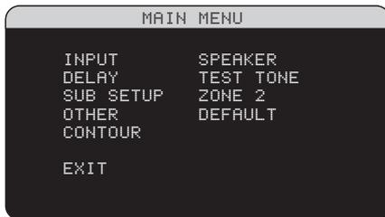
The MAIN MENU provides access to OSD screens for various configuration options. MAIN MENU is reached by pressing the ENTER button from the SYSTEM STATUS menu described above or from most other menus. To go to the desired menu, move the highlight using the UP/DOWN and +/- buttons on the remote and press the ENTER button. Press the MENU/OSD button on the remote to cancel the display and return to normal operation.
