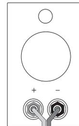
Figure 4 : Digital Input and 12 Volt Trigger Connections
