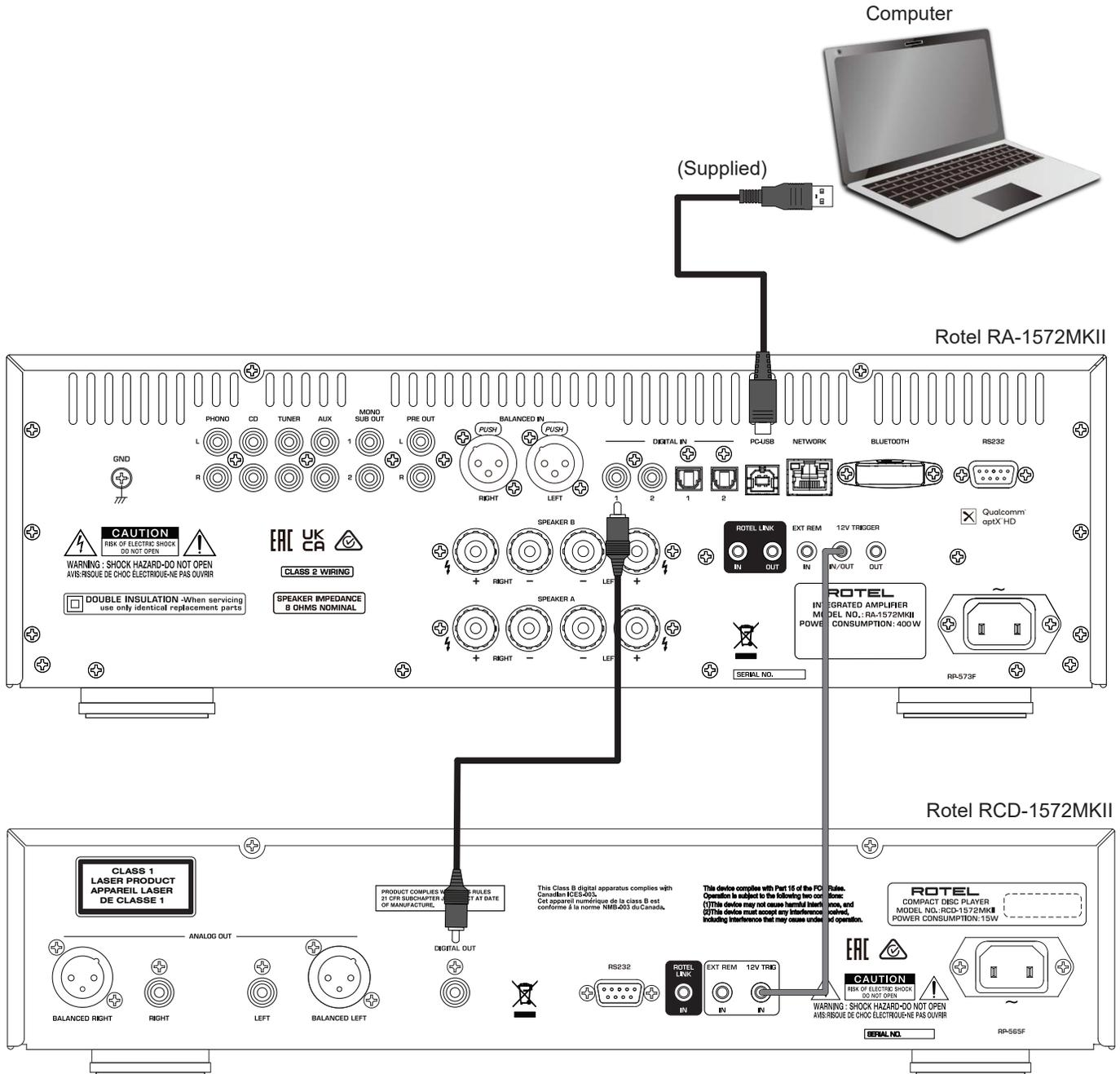
Figure 5 : **Balanced (XLR) Inputs Connection**
