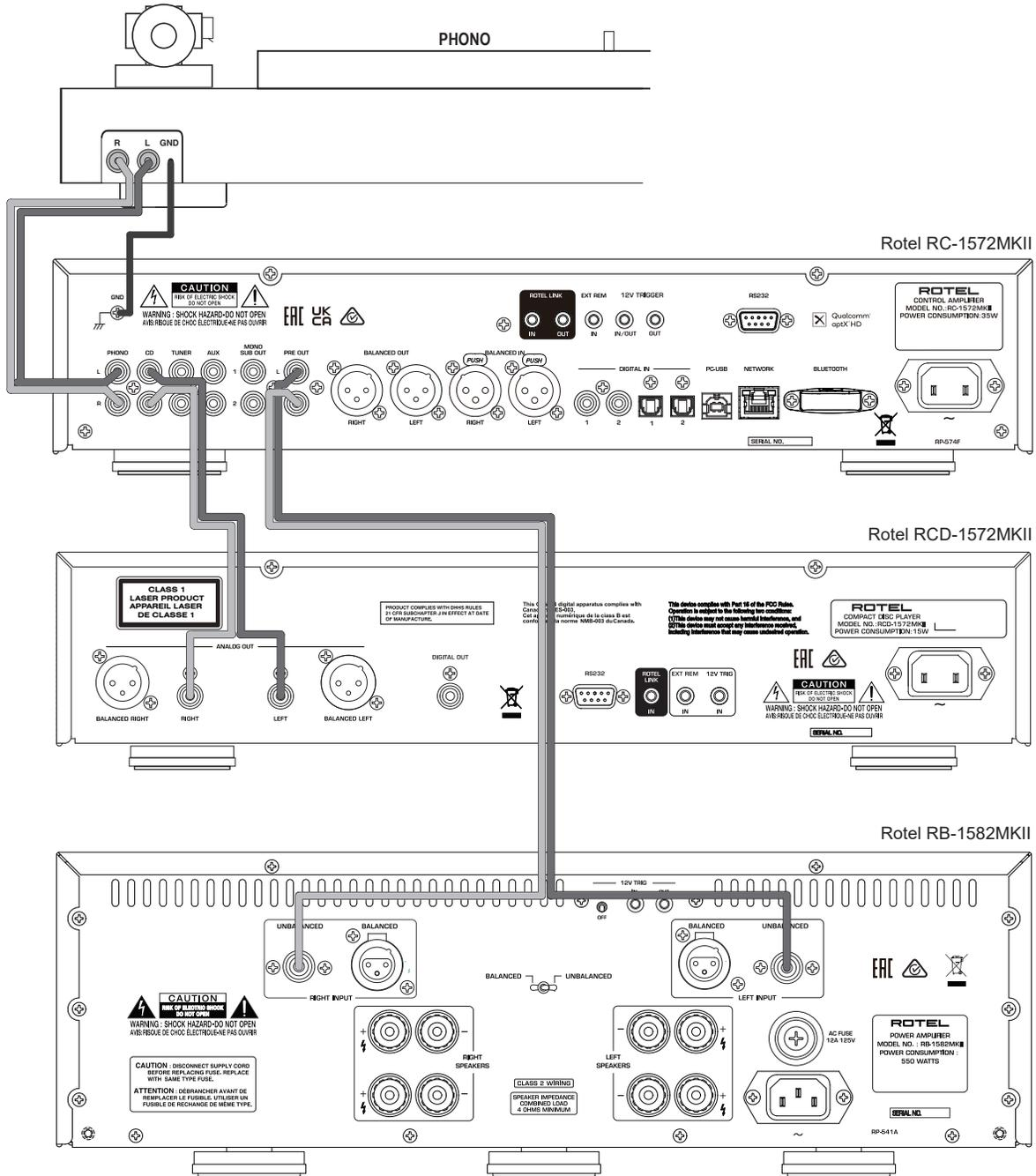
Figure 4 : **Balanced (XLR) Input and Output Connections**
