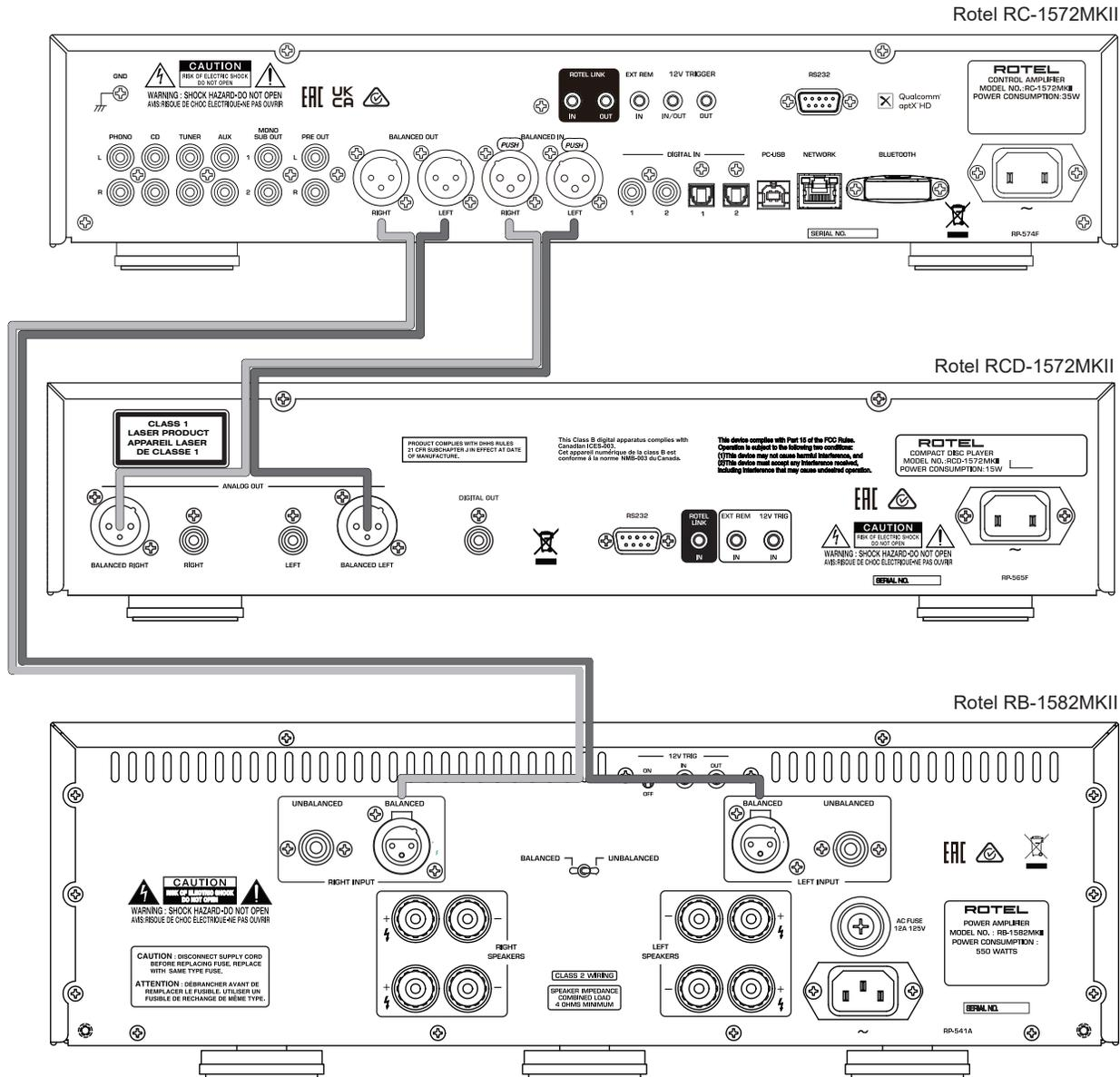
Figure 5 : Digital Input and 12 Volt Trigger Connections
