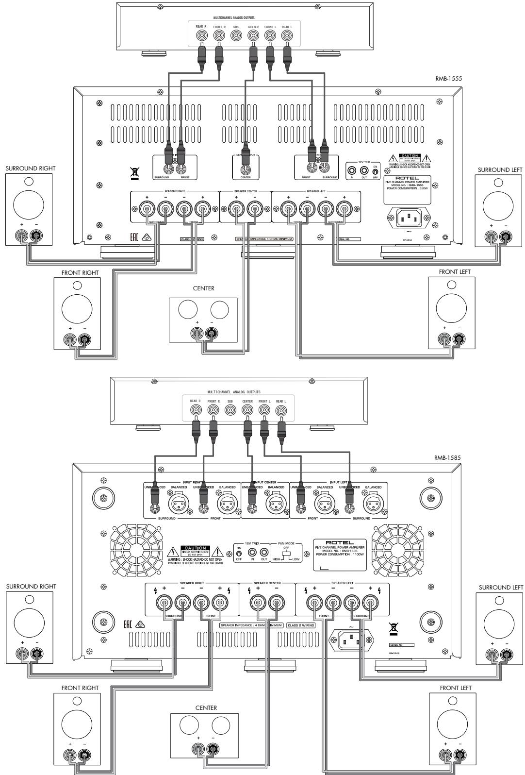
Figure 3: Balanced (XLR) Inputs
