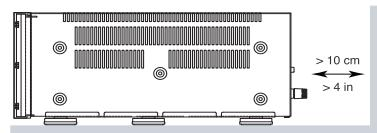
**WARNING:** The rear panel power cord connector is the mains power disconnect device. The device must be located in an open area that allows access to the cord connector.
